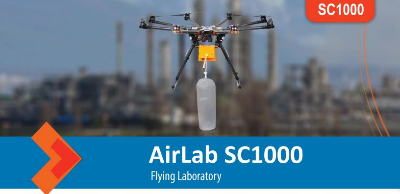
he SC1000 consists of a flying laboratory and a commercial drone. The SC1000 can be used to sample and analyze ambient air at heights of up to 150 meters above ground level that was previously impossible to accomplish. Air quality mapping, asset safety & performance monitoring, model verification, analysis of potentially dangerous sites are all made possible by this novel innovation.
